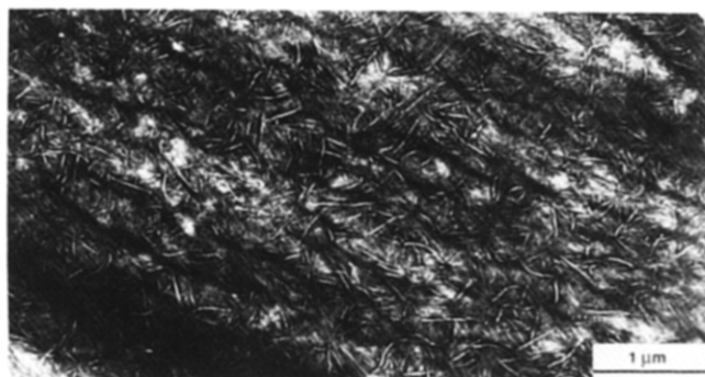
Figure 10 TEM micrograph of isothermally crystallized silane-grafted LLDPE
